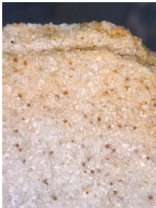
Figure 4: Oxidized pyrite (iron sulfide) grains generating a film of iron oxide on quartz grains. Note the rusty pigmentation near the weathered surface (top), but not deeper (bottom).
